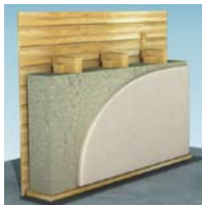
Banchage mur ossature bois
